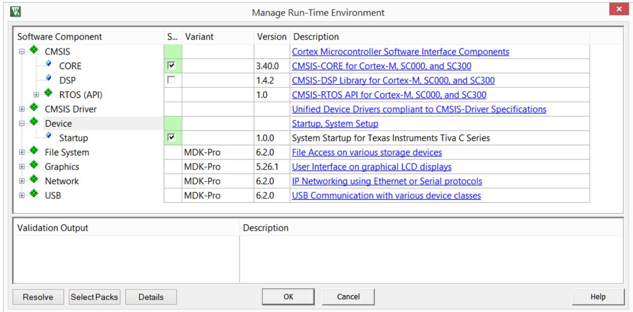
The projects in Keil v5 are created with an additional startup file named system\_TM4C123.c.
